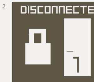
Flite Controller disconnected (requires pairing) and motor locked (requires arming).
